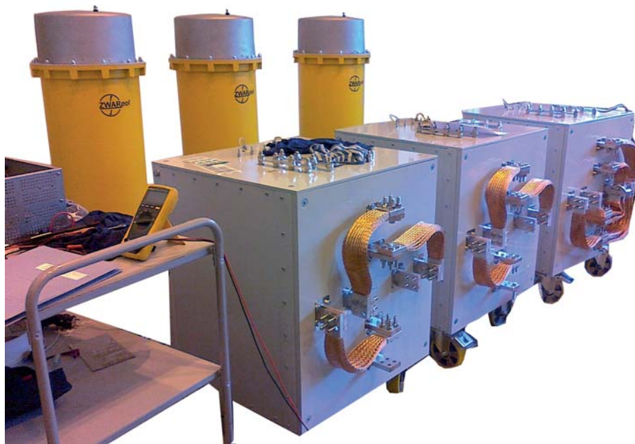
A set for high voltage three phase systems with TW25 and TRP10 transformers
