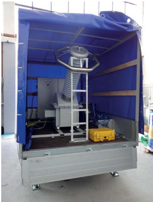
UP20-185 unit (20kVA, 185kV AC) adapted on a wagon
