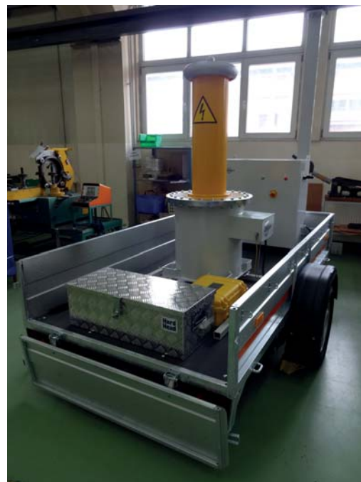
UP6J 100AC 130DC unit adapted on a wagon (a rectifier mounted on the top clamp of the transformer)
