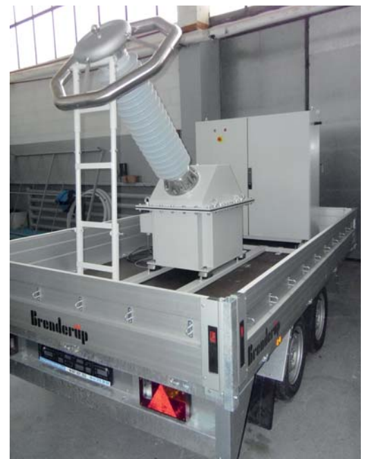
UP20-185 unit (20kVA, 185kV AC) adapted on a wagon
